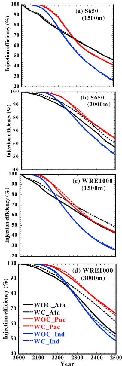
**Figure 1.** ISAM-2.5D simulated injection efficiency (defined as the ratio of the mass of injected carbon that remains in the ocean to the total injected carbon) for different ocean basins (Ata: Atlantic; Pac: Pacific; Ind: Indian). The calculations are done for with (WC) and without (WOC) climate change cases under S650 and WRE1000 CO<sub>2</sub> stabilization scenarios for injection depths of (a) and (c) 1500m and (b) and (d) 3000m.
